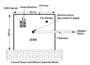
Figure 1: Diagram of RPI LSDS
