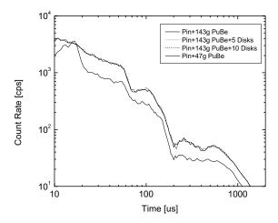
Figure 2: LSDS assay of (1) pin and small PuBe source and (2) pin, both PuBe sources, and 0, 5, and 10 HEU disks
