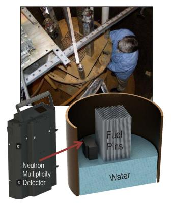
**Fig. 1.** Photograph of the RPI-RCF (*above*), and a Solidworks<sup>®</sup> simplified graphic rendering of the CaSPER measurement campaign at the RPI-RCF (*below*).
