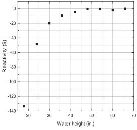
**Fig. 2.** Simulated reactivity worth curves for the RPI-RCF water height starting from the bottom of the fuel region.
