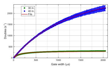
**Fig. 4.** Sample doubles fits from the LANL <sup>3</sup>He neutron multiplicity detector at different simulated water heights. Simulations were performed w/MCNP<sup>®</sup>6, and the fits were generated using Origin®.
