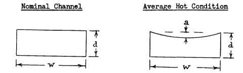
The reduction in flow area is estimated at 2/3 of the center deviation times the channel width.
