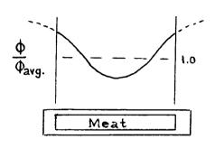
The water temperature rise up to any length along the channel is based upon progressive values of  $\varphi$  avg., or the average flux across the meat width. As the channel flow is well into the turbulent or high Reynolds number range, there are no local higher temperature rise regions in the main stream because of the
