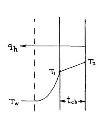
$$T_2 - T_w = q_h \left( \frac{1}{h_{ch}} + \frac{1}{h_f} \right)$$
