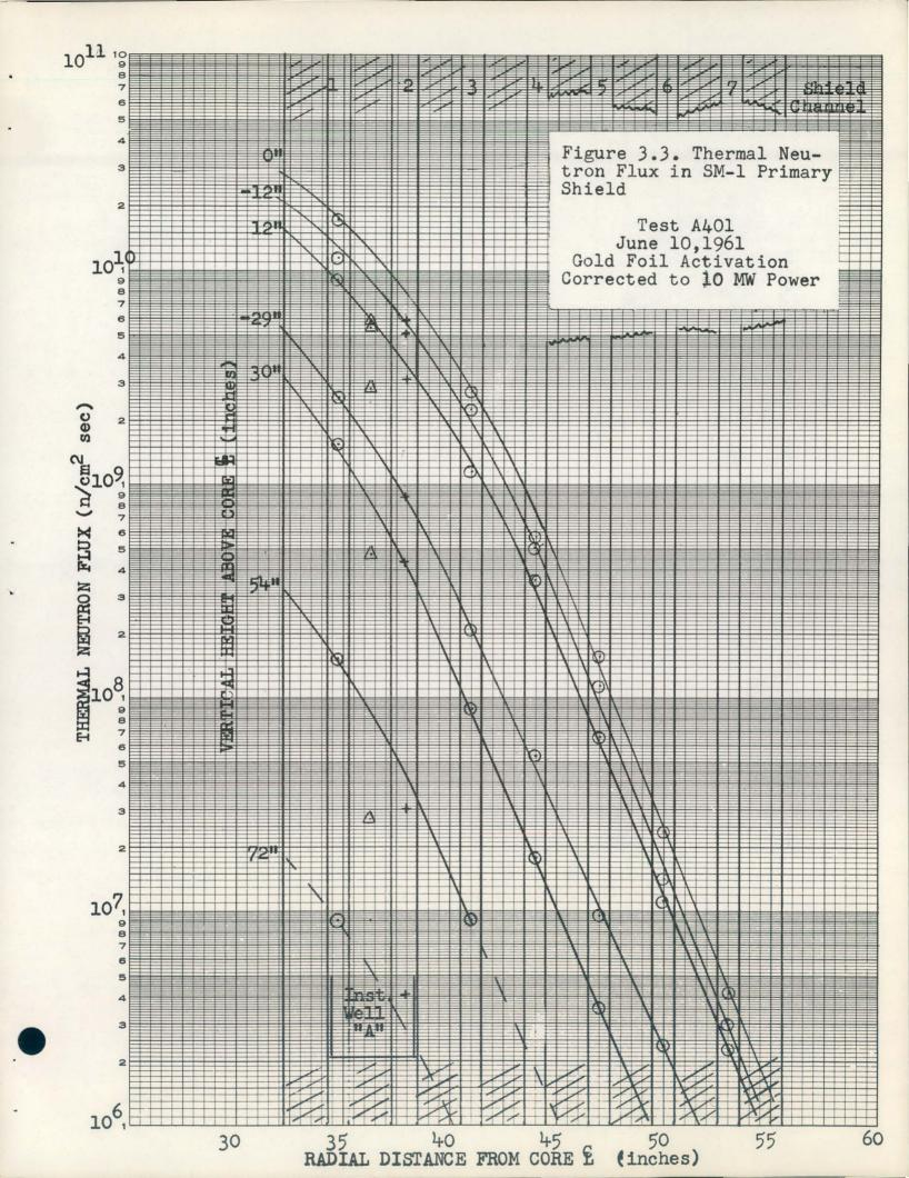
TABLE 3.3THERMAL NEUTRON FLUX THROUGH INNER SHIELD TANK AXIS
