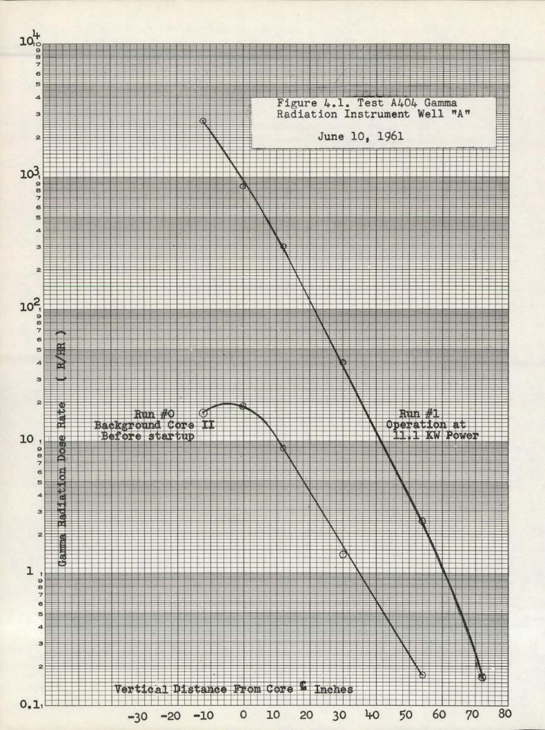
Strips of film were inserted in shield channels 1, 2, 3 and 4 and irradiated at 11.1 kw for 20 min, Run 1. The dose rates, converted to 10 Mw power level, are shown in Table 4.3 and Figs. 4.2 and 4.3.
