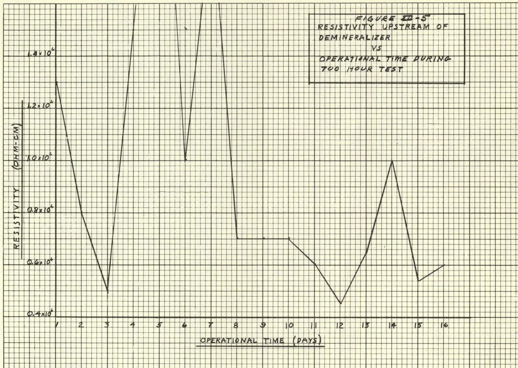
FIG. XII - 5 RESISTIVITY UPSTREAM OF DEMINERALIZER DURING 700 HOUR TEST
